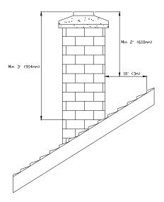
FIGURE 2.2 Minimum Height of the Chimney
